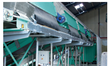
High effective system – conveyor takes the roughage to the mixer
