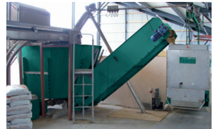
Fresh energy: The stationary mixer (MVM) and the feeder work hand-in-hand to make high-quality feed
