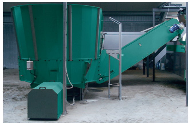
A minimum of work to fill the stationary mixer (example here: a 22 m 3 stationary mixer MVM22).
