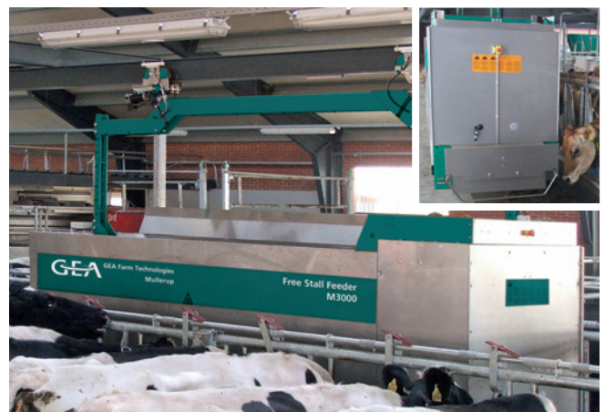
Busy supplier of feed: The computer-controlled, battery operated feeder serves up the feed for each animal group.
